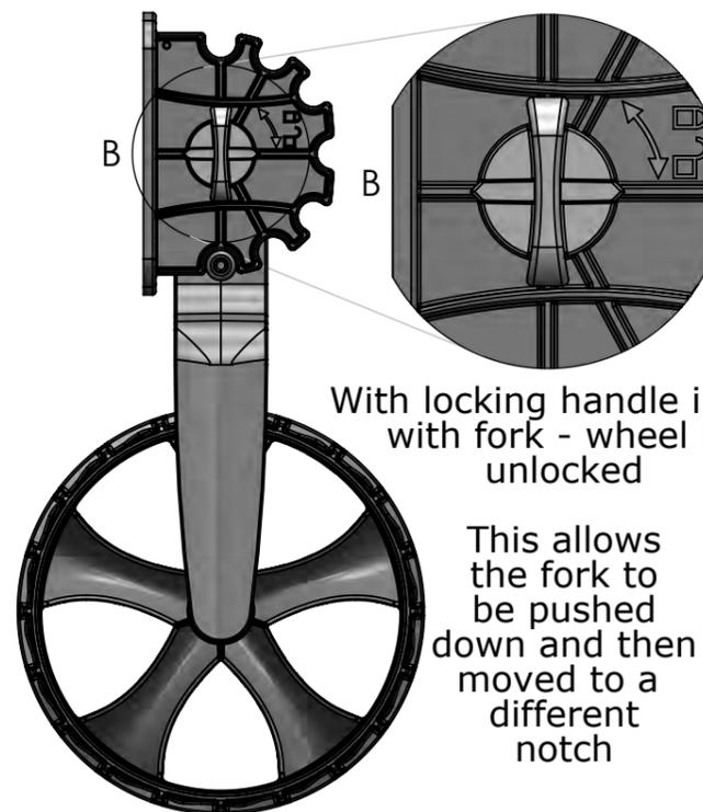
With locking handle in line with fork - wheel is unlocked
