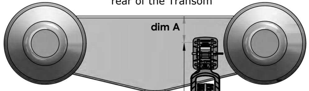
**1b** Position your assembled wheel bracket against the transom making sure the top of the wheel clears the bottom of the transom with fork in operating position
