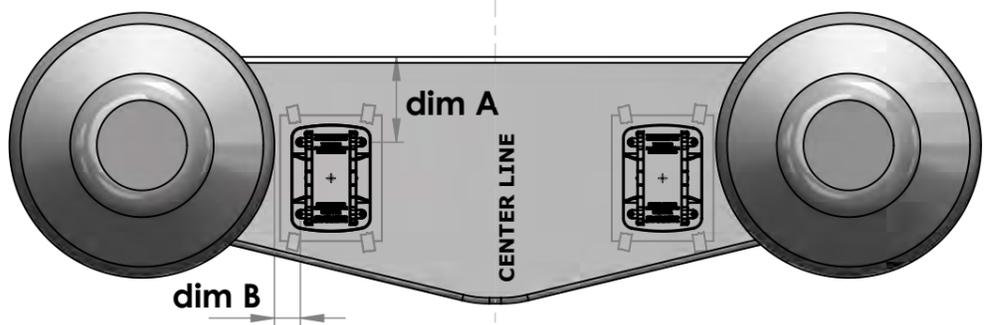
**2c** Check the distance **dim B** to the tube from the mounting holes - make sure there is at least 45mm (1.7") clear to allow space for the locking shaft
